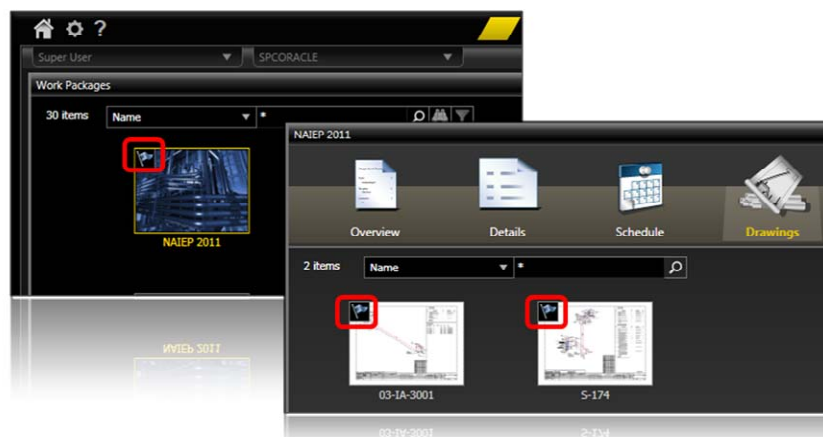
Figure 13: SmartPlant Construction enables automation of the change notice process, marking clearly the affected work packages.
