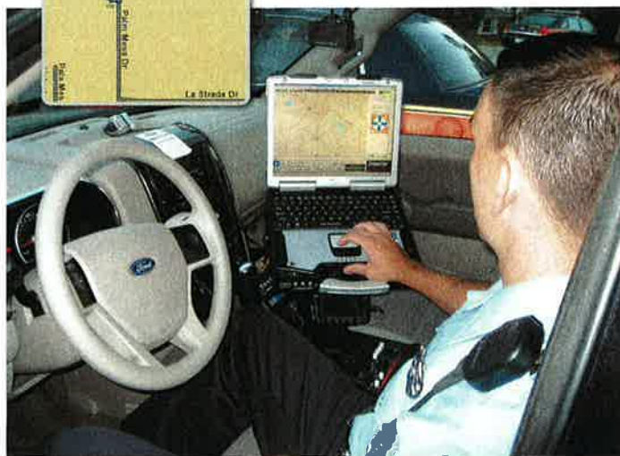
A Mobile Digital Communicator (MDC) System, like the one from Crimestar Corp. used by the Edwardsville, Ill., Police Department, dramatically boosts officer safety by being GPS and map enabled. A GPS receiver connected to the MDC allows transmission of real-time latitude and longitude coordinates back to CAD/Dispatch (top photo) so dispatchers and other MDC users can view field units spatially via the MDC or CAD map display. As a result, patrol units (bottom photo) and dispatchers can see at all times where units are and where events are occurring.
