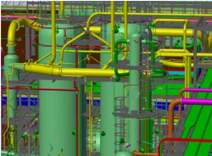
3d view of an intelligent SmartPlant model for a new polypropylene plant alongside a photograph of the completed facility. Images - Genpro.
