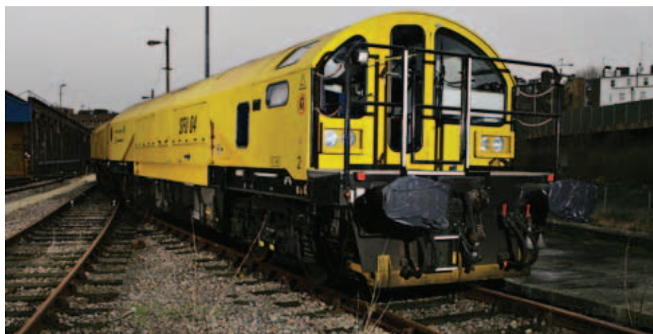
Rail milling train Tube Lines
